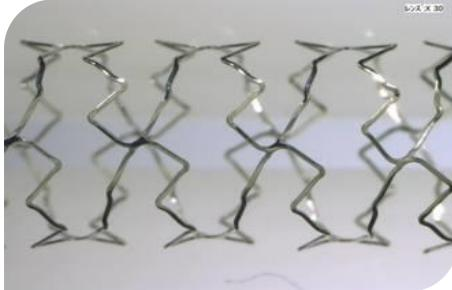
Over-expansion for each design was tested with successive post-dilations using first a  $5.0 \times 12$  mm non compliant balloon followed by a  $6.0 \times 15$  mm semi-compliant balloon with a pressure of 14 ATM for the largest designs.
